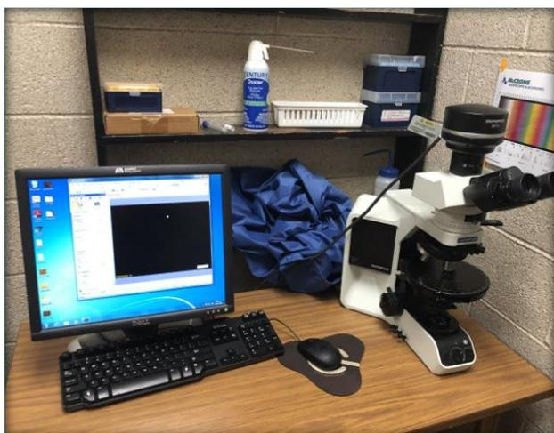
**FIGURE 2:** Olympus BX53 polarizing light microscope with computer monitor.
