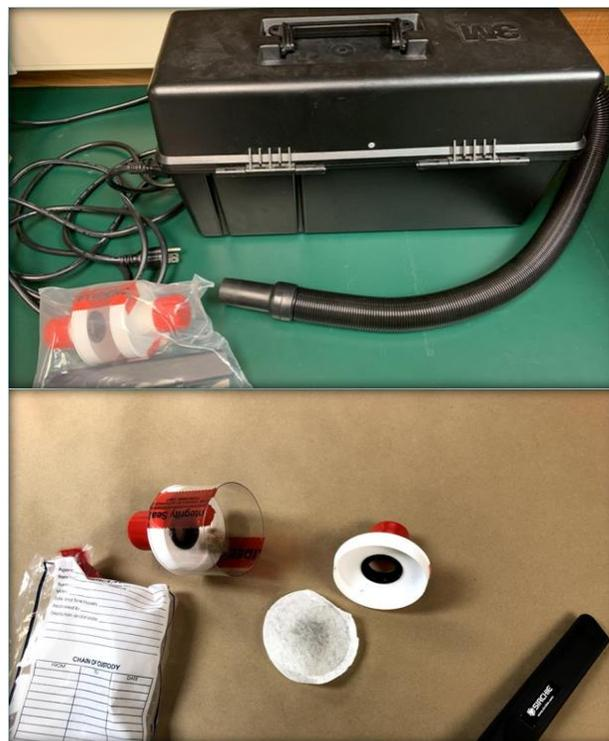
**FIGURE 1:** Top is a trace evidence vacuum; bottom is collection filter showing collected material on filter.
