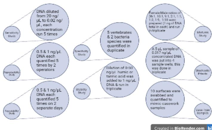
**FIGURE 1** Student-designed experimental design of Investigator Quantiplex Pro Kit validation conducted in Forensic Method Validation course.
