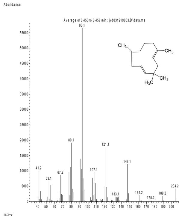
**FIGURE 10** Mass spectrum of beta-caryophyllene in alcohol extract (RT = 6.306 min)
