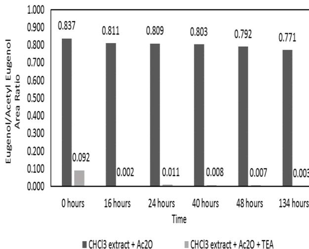
**FIGURE 14** Peak area ratios of eugenol to acetyl eugenol for chloroform extract + acetic anhydride and chloroform extract + acetic anhydride + triethylamine, over 134 hours
