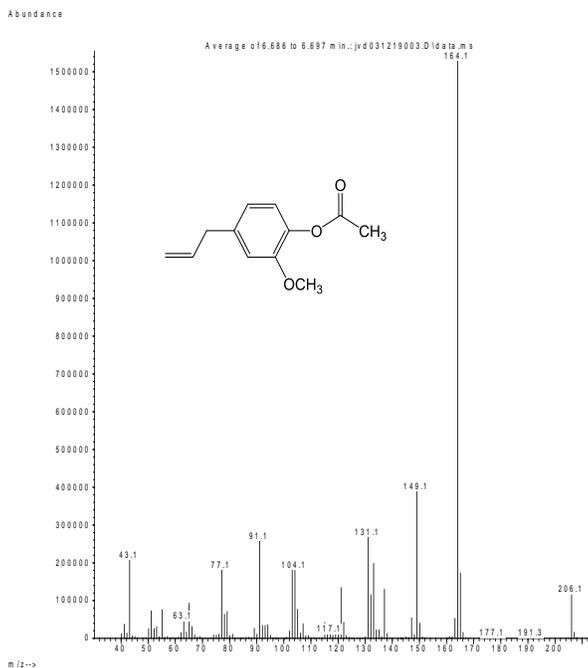
**FIGURE 8** Mass spectrum of eugenol in alcohol extract (RT=5.972 min)
