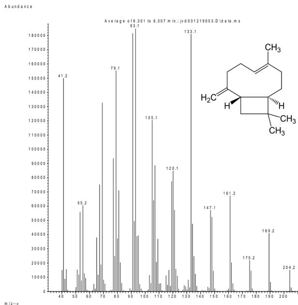
**FIGURE 12** Mass spectrum of caryophyllene oxide in alcohol extract (RT = 7.012 min).
