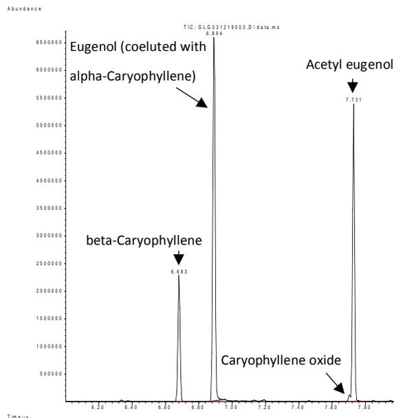
**FIGURE 13** GC-MS total ion chromatogram of alcoholic extract on HP-17 phase column
