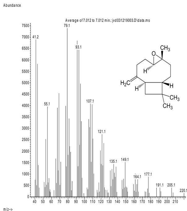
**FIGURE 11** Mass spectrum of alpha-caryophyllene in alcohol extract (RT = 6.457 min)
