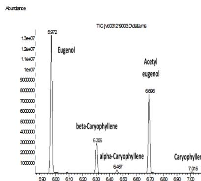
**FIGURE 7** GC-MS total ion chromatogram of alcohol extract on HP-5 phase column
