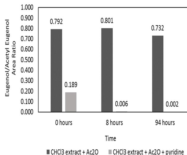
**FIGURE 15** Peak area ratios of eugenol to acetyl eugenol for chloroform extract + acetic anhydride and chloroform extract + acetic anhydride + pyridine, over 94 hours
