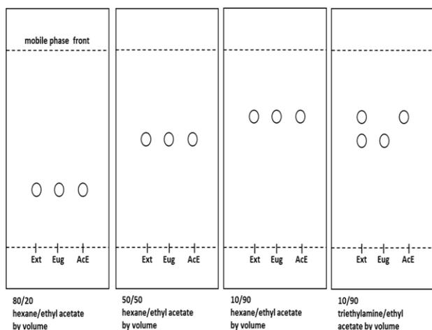
**FIGURE 5** TLC plates developed with hexane, ethyl acetate, and trimethylamine (Ext = alcoholic cloves extract, Eug = eugenol, AcE = acetyl eugenol).
