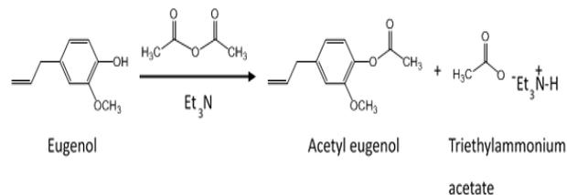
**FIGURE 3** Quantitative conversion of eugenol to acetyl eugenol via derivatization with acetic anhydride and triethylamine
